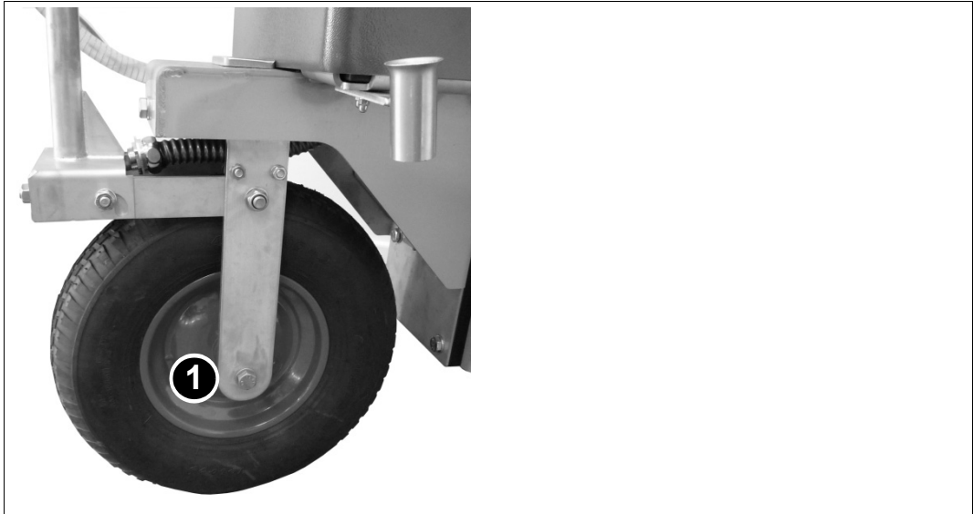
Figure 9/10: Changing the front wheel
