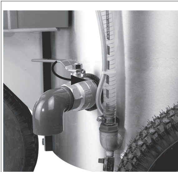
Figure 6/2: Manually removing the feed
